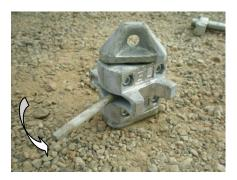
2. Insert Twist lock into top corner casting of shipping container with flat twist clamp at bottom.
